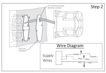
Step 2 - Install Silicone Grommet on J-Box Cover:
