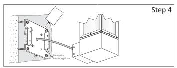
**Step 4** - Seal the Luminaire Mounting Plate:
