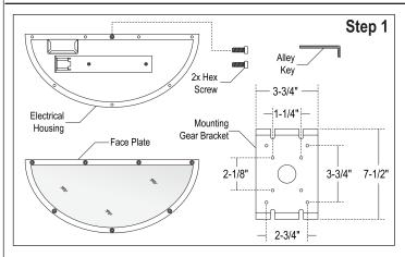
**Step 1 -** Remove Luminaire Parts for Installation:
