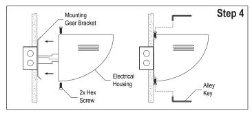
**Step 4 -** Installing Electrical Housing:
