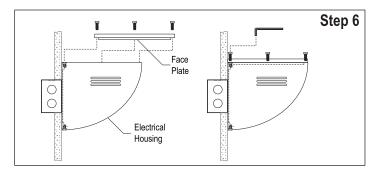
Step 6 - Installing Face Plate:
