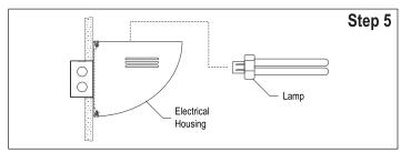
Step 5 - Installing Lamp:
