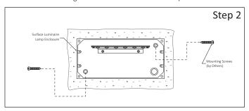
Step 2 - Install Luminaire Lamp Enclosure:
