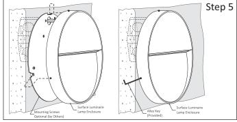
**Step 5 - Install Surface Mount Luminaire:**
