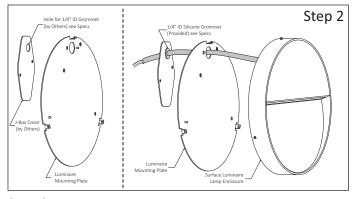
**Step 2** - Drill a Hole for Silicone Grommet on J-Box Cover:
