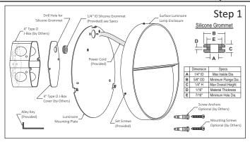
**Step 1** - Get Luminaire and proper Parts for Installation:
