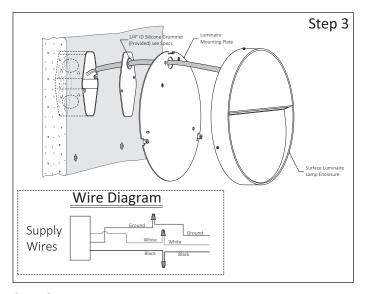
**Step 3** - Make Wiring Connections:
