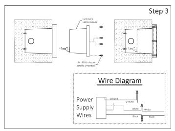
Step 3 - Install LED Enclosure / Make Wiring Connections:
