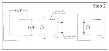
Step 2 - Install Luminaire CPX Box:
