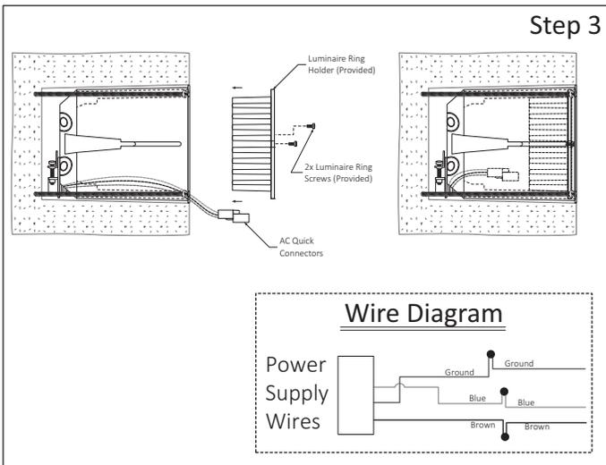
**Step 3 - Make Wiring Connections / Install Holder Ring:**
