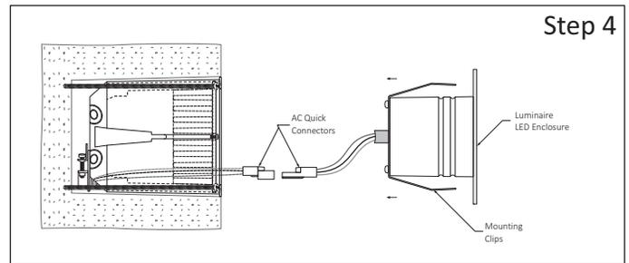
**Step 4 - Install Luminaire LED Enclosure:**
