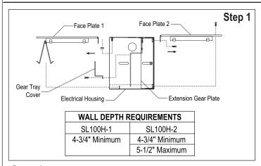
**Step 1 -** Remove Luminaire Parts for easy Installation:
