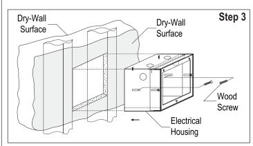
Step 3 - Install Electrical Housing:
