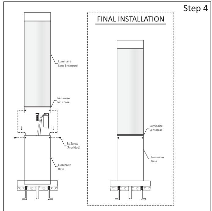
**Step 4 - Install Luminaire Lens Base:**
