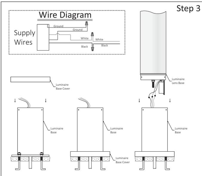
**Step 3 - Install Base Cover/Make Wiring Connections:**
