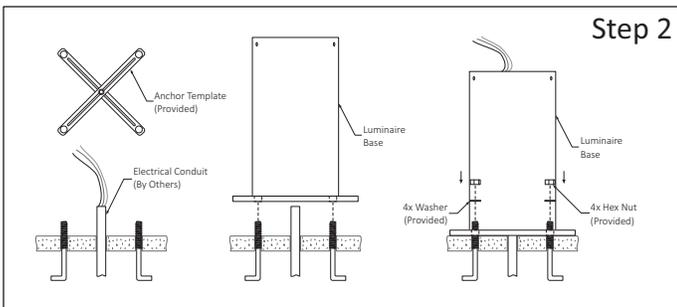
**Step 2 - Install Anchors Luminaire Base:**
