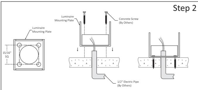
**Step 2 - Install Luminaire Mounting Plate:**
