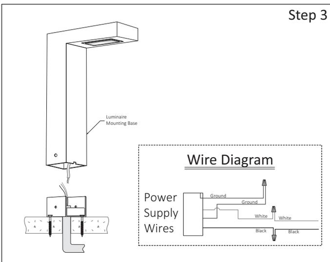
**Step 3 - Make Wiring Connections:**
