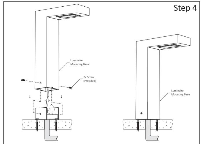
**Step 4 - Install Luminaire Mounting Base:**
