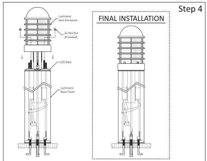
**Step 4 - Install Luminaire Lens Enclosure:**
