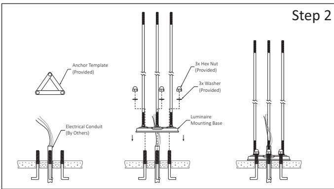
**Step 2 - Install Anchors Luminaire Mounting Base:**
