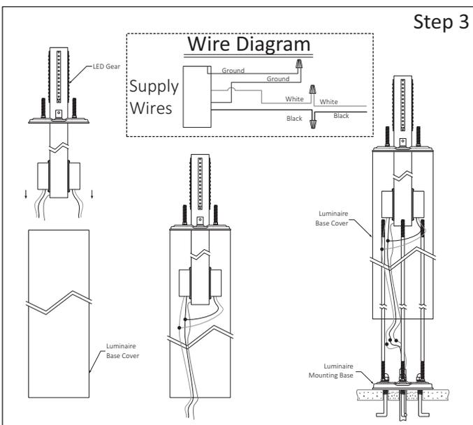
**Step 3 - Install Base Cover/Make Wiring Connections:**
