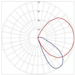
Maximum Candela = 72 Located At Horizontal Angle = 0, Vertical Angle = 37.5 # 1 - Vertical Plane Through Horizontal Angles (0 - 180) (Through Max. Cd.) # 2 - Horizontal Cone Through Vertical Angle (37.5) (Through Max. Cd.)
