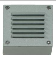
**Description :** ADA surface mounted luminaire for low level illumination application. Constructed from low copper aluminum die-cast. Suitable for wet locations. Tempered frosted glass diffuser. High corrosion resistant polyester powder coat finish. Vandal resistant stainless steel screws. Specify any RAL. ETL listed for wet locations.
