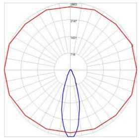
Maximum Candela = 2862.6 Located At Horizontal Angle = 0, Vertical Angle = 2.5 # 1 - Vertical Plane Through Horizontal Angles (0 - 180) (Through Max. Cd.) # 2 - Horizontal Cone Through Vertical Angle (2.5) (Through Max. Cd.)
